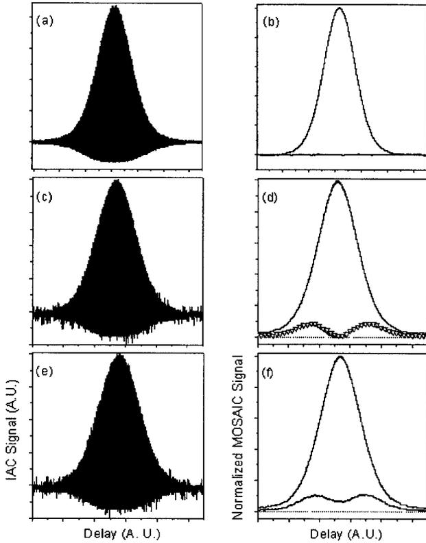
Fig. 1. Experimentally obtained IAC traces of an (a) unchirped pulse, (c) a chirped pulse, and (e) a chirped pulse with distortion. The distortion is produced by misaligning the autocorrelator. Corresponding MOSAIC maximum and minimum envelopes are shown in (b), (d), and (f). The corrected minimum envelope of the MOSAIC is depicted in (d) with triangles.
