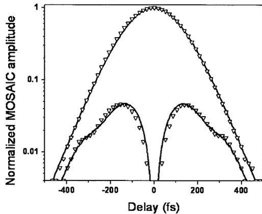
Fig. 3. Semilog plot of the experimental data (triangles) and fit (solid curves) that reveal high-order components of chirp on a 120 fs Ti:sapphire laser pulse.
