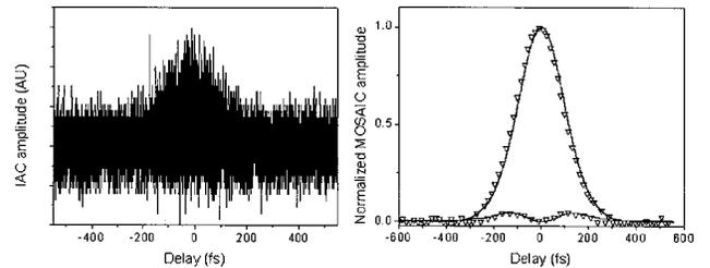
Fig. 2. Left, single IAC trace just above the noise level. Right, averaged MOSAIC waveform produced after acquiring 1200 noisy IAC traces (triangles); the chirp of the same pulse obtained with negligible noise is reproduced (solid curve).
