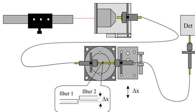
**Figure 6:** Experimental setup to measure coupling losses between to multi-mode fibers.
