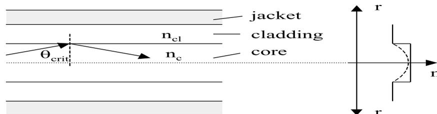
**Figure 1:** Layout of an optical step-index fiber. The refractive index profile for a graded-index fiber is shown as a dashed line for comparison.
