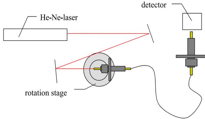
**Figure 3:** Experimental setup to measure the NA of a multimode fiber.
