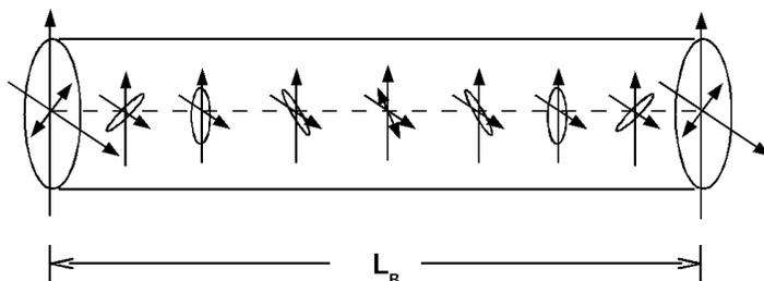
**Figure 5:** Illustration of polarization state change in a fiber and its relation to the beat length.
