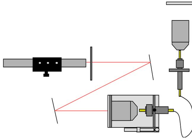
**Figure 8:** Experimental setup to observe mode patterns produced in a single mode fiber.
