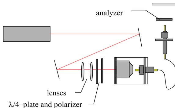
**Figure 7:** Experimental setup to study a polarization-preserving fiber.
