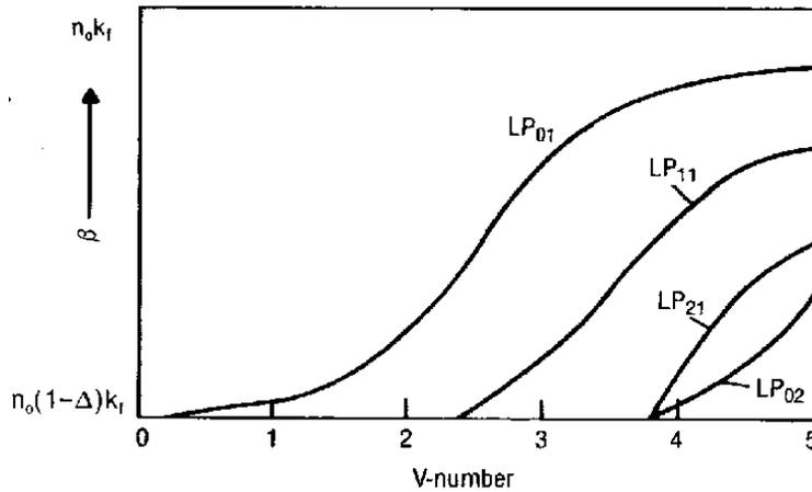
**Figure 4:** Propagation constant as a function of the V-number.  $k_f = 2\pi/\lambda_0$
